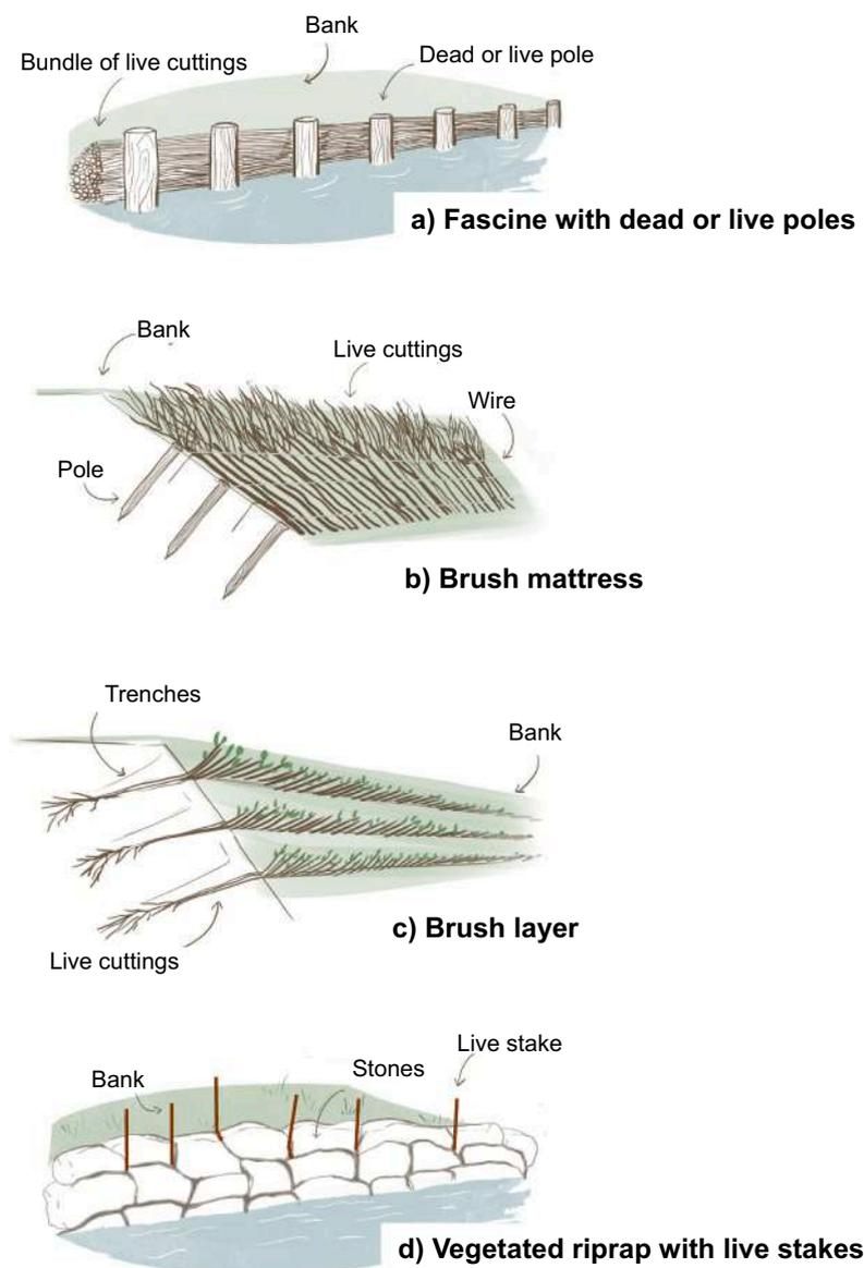
Fig. 2. Illustrations of four SWBE techniques, a: Fascine, b: brush mattress, c: brush layer, d: vegetated riprap.
